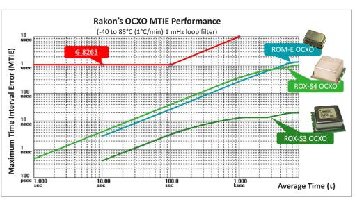
technologies require tight phase accuracies ( $\pm 1.5~\mu s$ ) and applications like Location Based Services (LBS) are driving accuracy requirements to even more stringent values ( $^{\sim}500~n s$ ). ROX2522S4 devices provides the performance of traditional Stratum 3E discrete OCXO performances. Footprint compatible ROX2522S3 products improve the performance one magnitude, introducing 1 ppb temperature stability and 0.2 ppb/day ageing performance.
