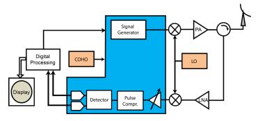
This new level of integration into a so called Digital Sub-System (DSS) simplifies the global radar architecture, thus reducing mechanical size (less racks), cost and maintenance.
